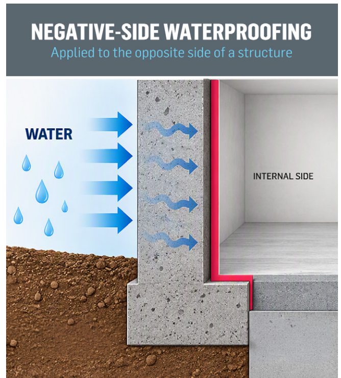
Pic 2. Negative-side waterproofing.
