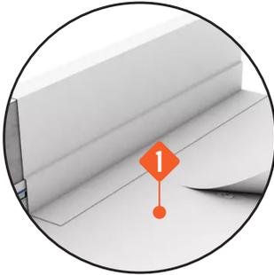
1. Waterproofing membrane: **FLAGON EP/PR ENERGY PLUS**
