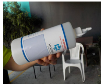
3. Shake for 2 minutes. For quicker dry times induct for 3-5 minutes and then shake and apply.
